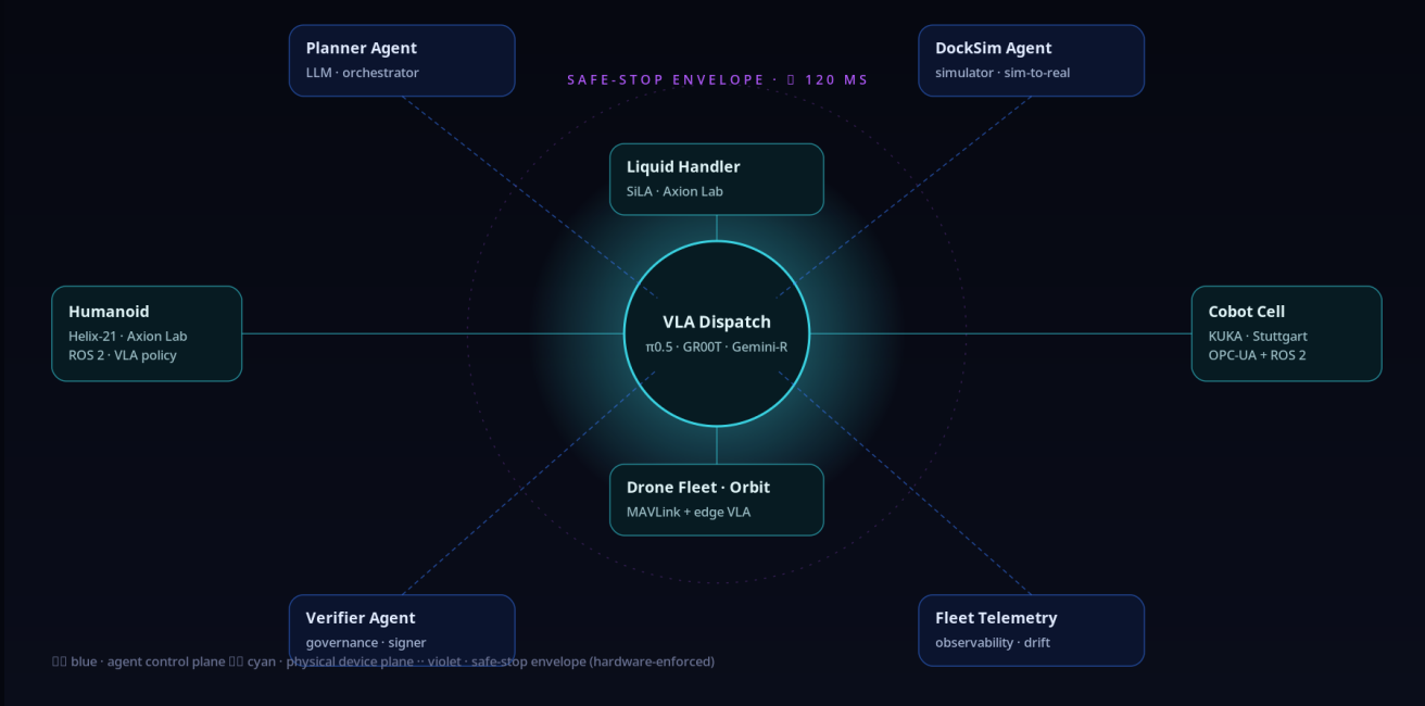
Figure 4 — Physical AI Bridge Topology. Blue: agent control-plane nodes (Planner, DockSim, Verifier, Fleet Telemetry). Cyan: physical device nodes (Humanoid, Cobot Cell, Liquid Handler, Drone Fleet). Violet dashed circle: safe-stop envelope ( \leq 120 ms hardware-enforced).
